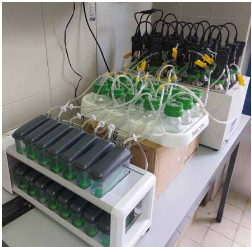
Laboratory instrumentation used for Biomethane Potential tests (Gas Endeavour, BPC Instruments)
